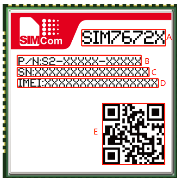
Figure 34: Label information for SIM7672X
